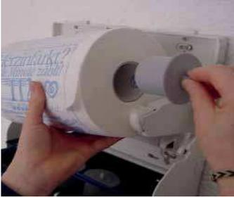
To load the first roll plug the plastic holders into both ends of the roll and then lay the roll into the dispenser so both pins locate into the paper roll cradles. The roll should be ready to dispense towards you from the top of the roll.
