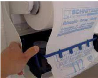
With the blue lever on the left side, raise the front paper guide with paper feed through.
