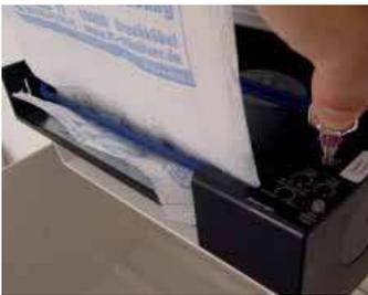
Press the button labelled "Manual operation" and the paper is automatically pulled in and dispensed from the device.
