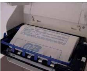
For this purpose, remove the old roll from the upper cradle and insert into the lower cradle. Push down all the way. The paper guide is then raised forward automatically.
