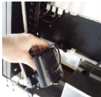
8. Lift out the gearbox
