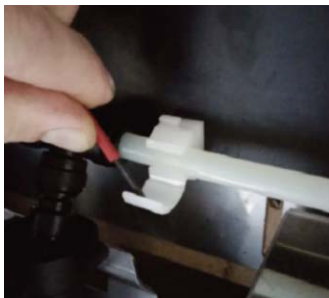
3. Open the pipe clips at the tee
