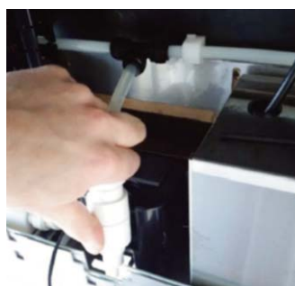
4. Remove pump from gearbox
