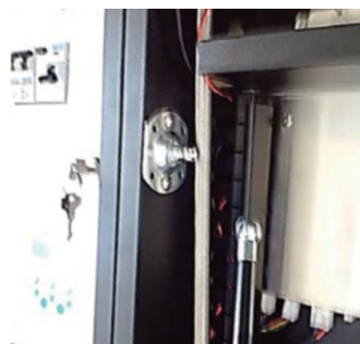
5. Pop bottom of strut off the bracket
