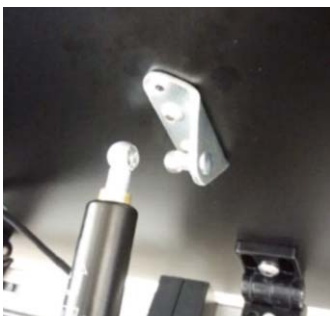
4. Pop top of strut off the bracket
