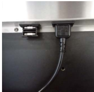
1. Slide open the fuse holder
