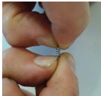
7. Catch 2 coils & stretch spring slightly
