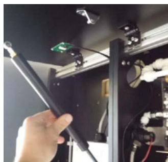
Support the strut and lower it
