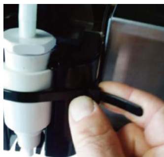
3. Undo cable tie restraining pump
