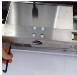
4. Undo the 2nd T30V retaining screw
