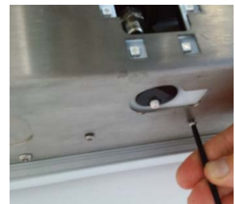
5. Undo the 2 x T20V retaining screws
