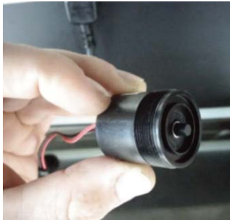
4. Remove diaphragm from solenoid
