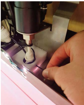
1. First undo the grub screw which hold the sensor in place
