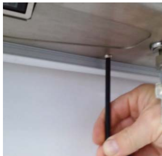
3. Undo the 1st T30V retaining screw
