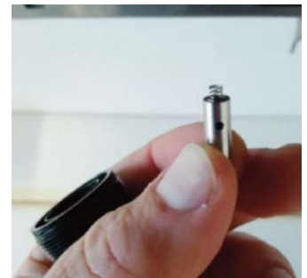
8. Replace spring in pin solenoid holding up
