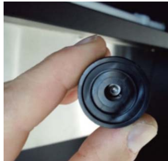
Spring fallen onto its side
