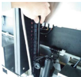
Refit the cover to the conduit
