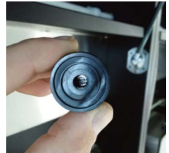
5. Remove pin and check spring
