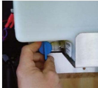
1. Turn off the soap supply at the tank / reservoir
