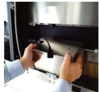
5. Lift out the dryer unit
