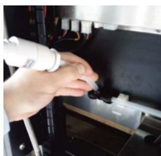
7. Push new pump firmly into tee
