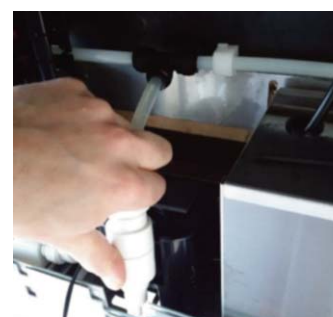
8. Fit new pump into gearbox
