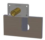
Pass conduit and conduit adapter through the Ø40mm hole
