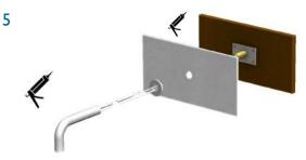
Fit Splashback with adhesive (or other fixing method as required) leaving mounting assembly protruding (thru Ø21mm hole) ready for Inform Tap Installation (See separate installation guide).
