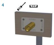
Fix the Wall Mounting Kit assembly with 4 screws supplied. IMPORTANT: Slot to be on underside of tail. Ensure wall plate is level as this dictates tap angle and rotation.
