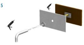
Fit Splashback with adhesive (or other fixing method as required) leaving mounting assembly protruding (thru Ø25mm hole) ready for Inform Tap Installation (See separate installation guide).
