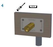
Fix the Wall Mounting Kit assembly with 4 screws supplied. IMPORTANT: Slot to be on underside of tail. Ensure wall plate is level as this dictates tap angle and rotation.
