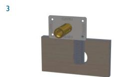
Pass conduit and conduit adapter through the Ø40mm hole
