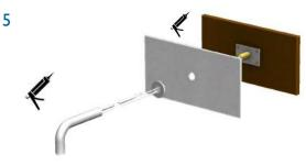
Fit Splashback with adhesive (or other fixing method as required) leaving mounting assembly protruding (thru Ø21mm hole) ready for Inform Tap Installation (See separate installation guide).
