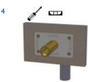
Fix the Wall Mounting Kit assembly with 4 screws supplied. IMPORTANT: Slot to be on underside of tail. Ensure wall plate is level as this dictates tap angle and rotation.
