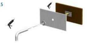
Fit Splashback with adhesive (or other fixing method as required) leaving mounting assembly protruding (thru Ø25mm hole) ready for Inform Tap Installation (See separate installation guide).
