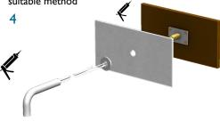
Fit Splashback with adhesive (or other fixing method as required) leaving mounting assembly protruding (Ø21min hole)
