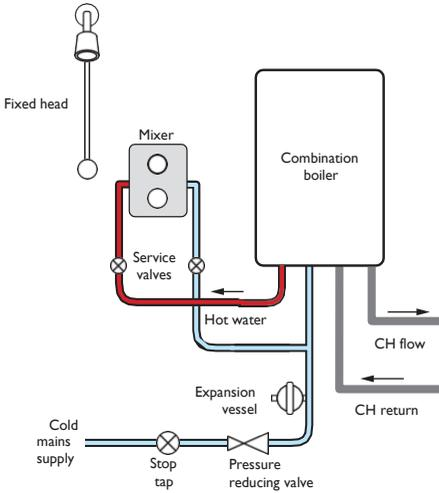
**Instantaneous gas-heated systems, e.g. combination boilers (fig.4)**
