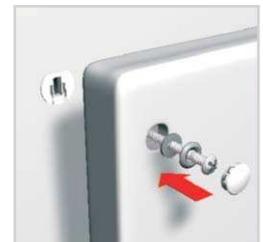
**5** Align and engage the fixing bolt in the threaded toggle bar with washers engaged. The flat fender washer is to be inserted underneath the finishing washer. Finally, insert the snap-fit plastic covers in each fixing port.
