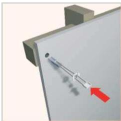
**1** Mark out and drill fixing holes. Insert toggle.
