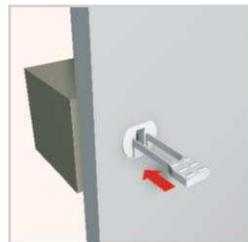
**3** Push the integral disc along the toggle to make a snug purchase on the wall face. The toggle strands are ratched to hold the disc in place.
