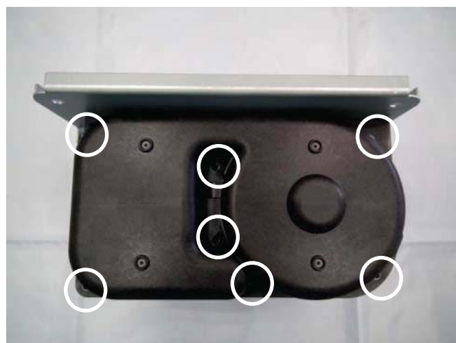
2. Loosen the fixing screws of the blower and remove the blower housing.
