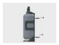
4 Connect the quick connection fitting to the soap dispenser pump. Make sure it is firmly plugged in.
